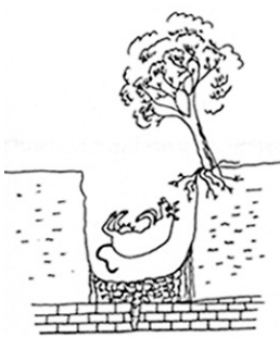
Sketch above depicts development of a cover collapse sinkhole by piping of soil particles and the formation of a soil arch which fails totally.
